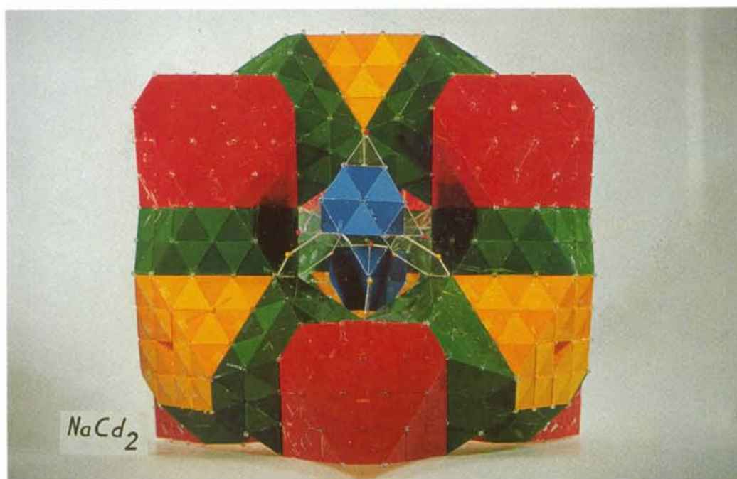
Fig. 2. The structure of \text{NaCd}_2 . The building block (4, 3, 1) consists of one red or yellow unit and four half green units. The blue Friauf polyhedron + red balls constitute the (3, 0) building block.
